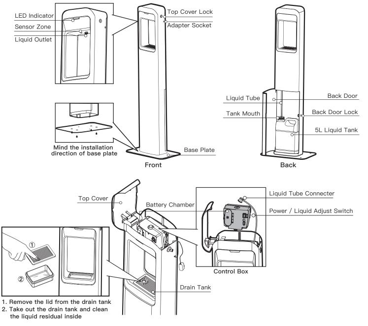
1 Place the product horizontally, put the base plate corresponding to the position of 2 guide posts at the bottom of product.
